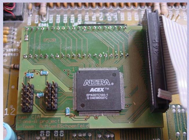
This single FPGA implements both of the Amiga's Complex Interface Adaptor (CIA) chips.
